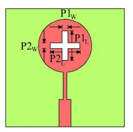
Fig. 1 Top view configuration of CCMSA
