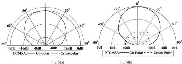
Fig. 5 Typical co-polar and cross-polar radiation pattern of CCMSA and PTCMSA measured at 3 GHz and 2.62 GHz respectively.
