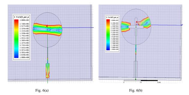
Fig. 6 E-plane field distribution of CCMSA and PTCMSA observed at  $f_r$  and  $f_{rl}$  respectively
